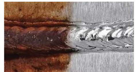
*Failure to clean and passivate the weld can have a serious impact on the lifecycle of the weld - such as corrosion, pitting, crevice corrosion and fatigue.*
