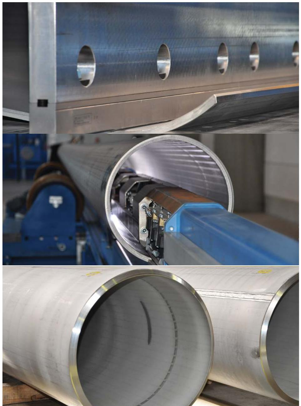
*Pipe fabrication at Sosta: (1) forming on the press brake, (2) welding the inside and (3) finished pipes. Sosta manufactures welded stainless steel pipe for the oil and gas market. Its pipes are used in gas exploration and liquefied natural gas plants and terminals.*
