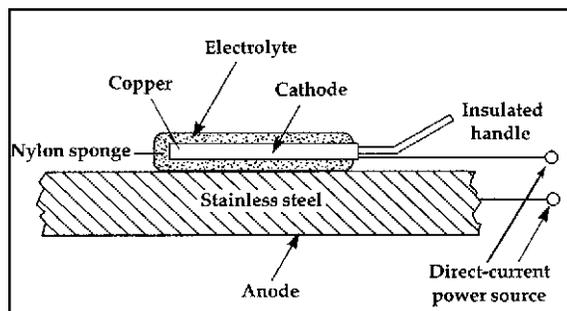
Localized electrocleaning of heat tint from the surface of stainless steel can be performed with a simple tool such as the one shown here.
