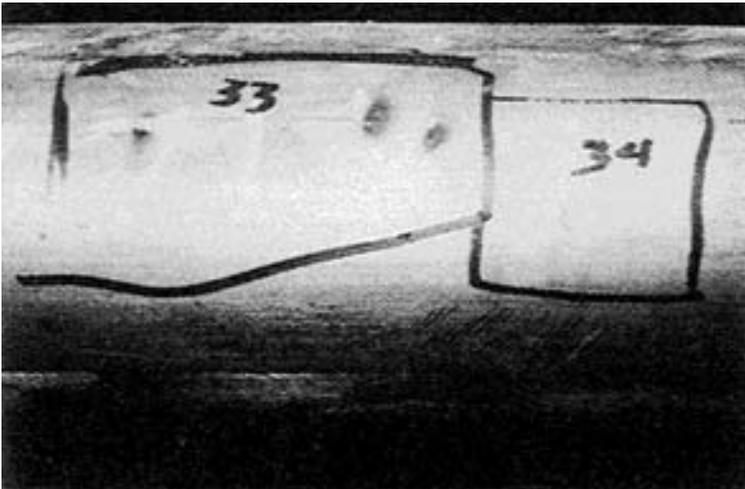
*Crevice corrosion can be initiated by deep scratches, top and by paint and other markings, such as those made by a marking crayon, bottom. Removal of the markings would have prevented the corrosion.*
