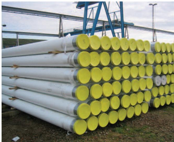
*Welded duplex line pipe manufactured by Sosta. These pipes are used for transportation of high-temperature, corrosive gas from the wellhead to the processing plant. Sosta has supplied over 300km of this pipe to oil projects in Oman, Nigeria, Germany and Pakistan. The pipes are manufactured in accordance with API5L from duplex grade UNS S31803 (2205). These pipes are mostly coated with polypropylene coating.*
