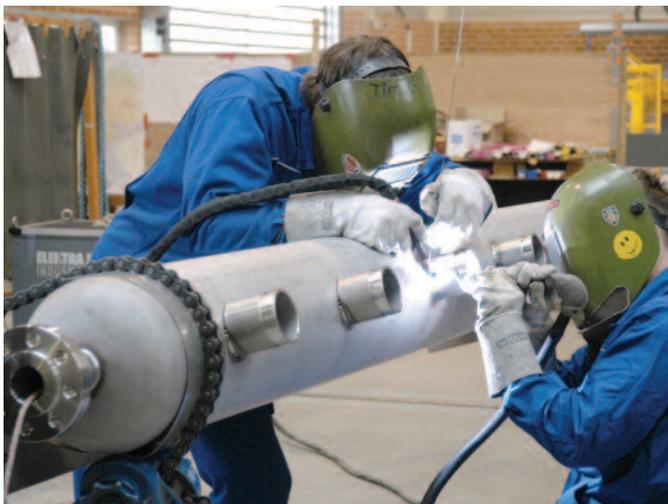
Prefabrication of the piping components for a seawater desalination plant. Photo © H. BUTTING GmbH & Co. KG.
