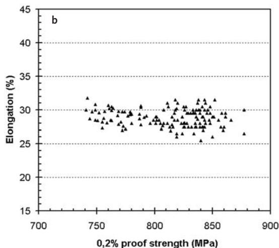
Fig. 3. Tensile properties of SAF 3207 HD tube materials: (a) 0.2% proof strength and tensile strength versus temperature, (b) elongation versus 0.2% proof strength.
