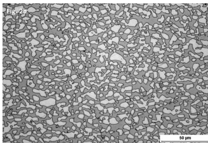
Fig. 2. Microstructure of Sandvik SAF 3207 HD tube material with a dimension of 14.7 x 1 mm. The white phase is austenite, and the grey phase is ferrite: (a) longitudinal direction, (b) transversal direction.
