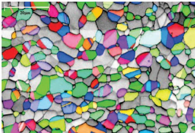
Fig. 4. Grain structure in a SAF 3207 HD umbilical tube with a dimension of 14.7 x 1 mm. Color grains are austenitic phase (3.6  $\mu\text{m}$ ), and grey grains are ferritic phase (5.1  $\mu\text{m}$ ).
