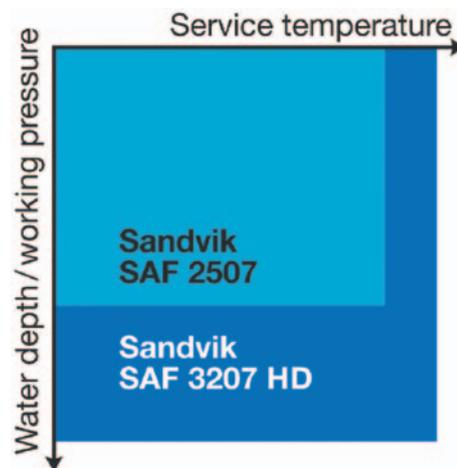
Fig. 6. Problem solution with Sandvik SAF 3207 HD tube materials
