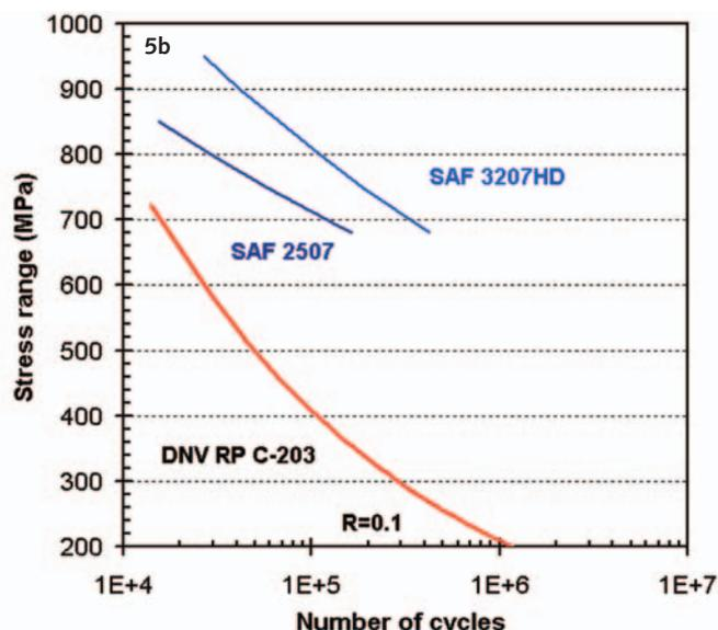
Fig. 5 Fatigue properties of Sandvik SAF 3207 HD tube materials: (a) LCF in air, tubes: 14.7 x 1 mm, (b) HCF in air, tubes: 14.7 x 1 mm, (c) HCF in air and in synthetic sea water, tubes: 21.25 x 1.05 mm, (d) welded material, tubes: 14.7 x 1 mm. All HCF curves have a survival probability of 97.5%.
