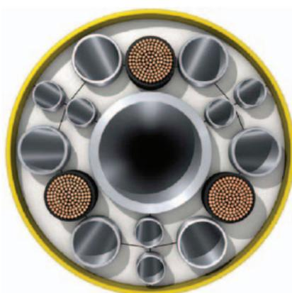
Fig. 1. Schematic section diagram of a subsea umbilical.
