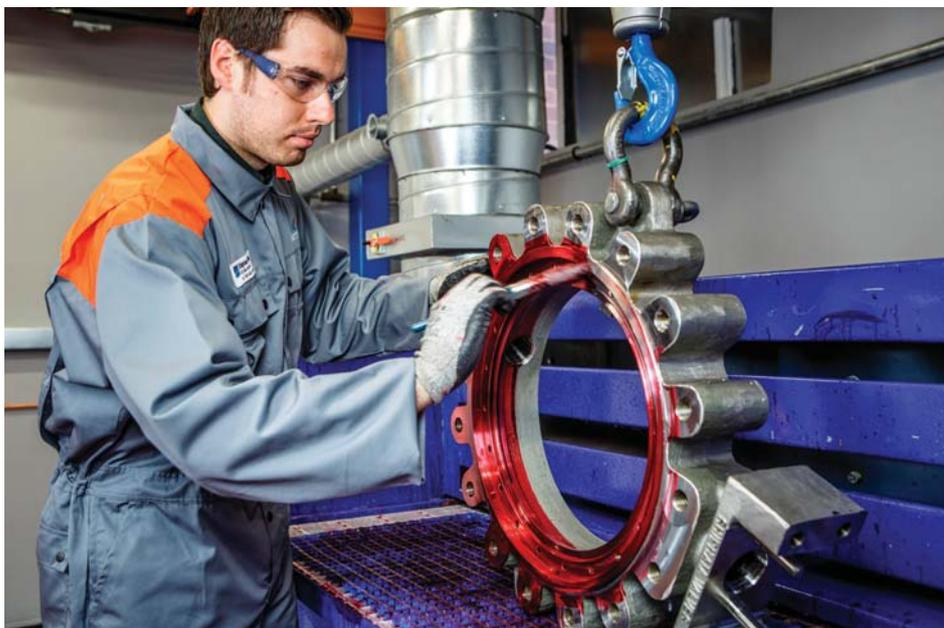
*A duplex butterfly valve undergoing liquid penetrant inspection to check integrity of casting quality at Wärtsilä Shipman Valves.*
