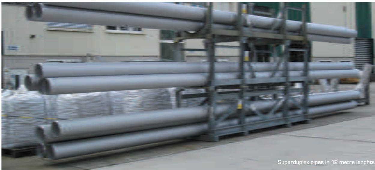
Superduplex pipes in 12 metre lengths
