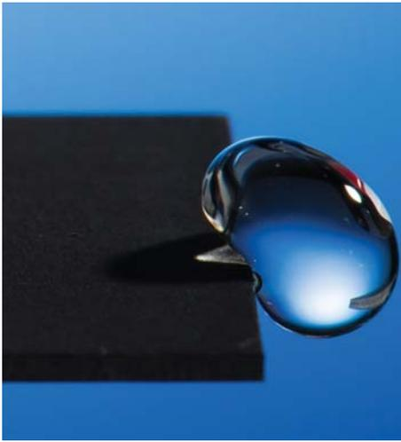
*The light absorption and super-hydrophobic properties of the laser treated steel could make it ideal for corrosion resistant, self-cleaning solar panels. Photo: J. Adam Fenster, University of Rochester*
