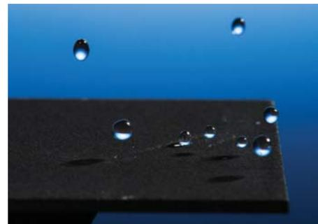
Professor Chunlei Guo has developed a technique that uses lasers to render materials hydrophobic, illustrated in these images of water droplets bouncing off a treated sample. Photos: J. Adam Fenster, University of Rochester
