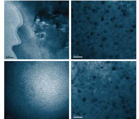
Transmission electron microscopy image showing different levels of crystallinity embedded in the amorphous matrix of the alloy. Photo: Jacobs School of Engineering/UC San Diego
