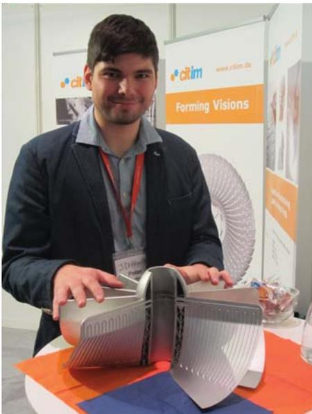
Laser beam melting is a powerful additive manufacturing technique, explains citim’s Peter Böttner. Giving an example, he indicates that this particular 3D structure was printed with channels inside the blades for cooling and boasts a lattice-work arrangement for a high-strength, low-weight central shaft. Try making something like this using conventional techniques!
