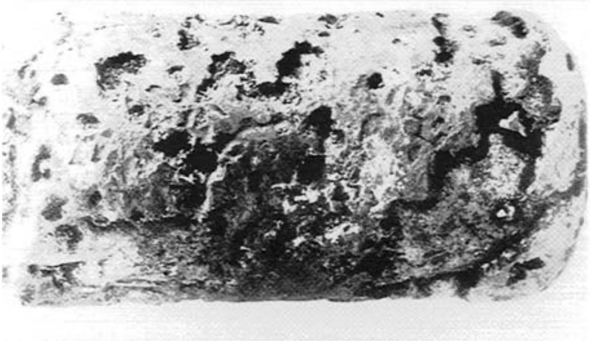
**Fig. 9 Pitting in horizontal weld seam of type 316 tank - MIC (Kobrin)**
